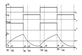
Fig 8 Waveform of series resonant half bridge inverter
