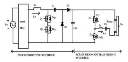
Fig 3 Pseudoboost electronic ballast for CFL
