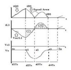
Fig 6 Theoretical waveform of Pseudoboost converter during negative half cycle
