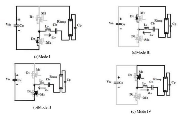
Fig 7 Modes of operation of series resonant half bridge inverter
